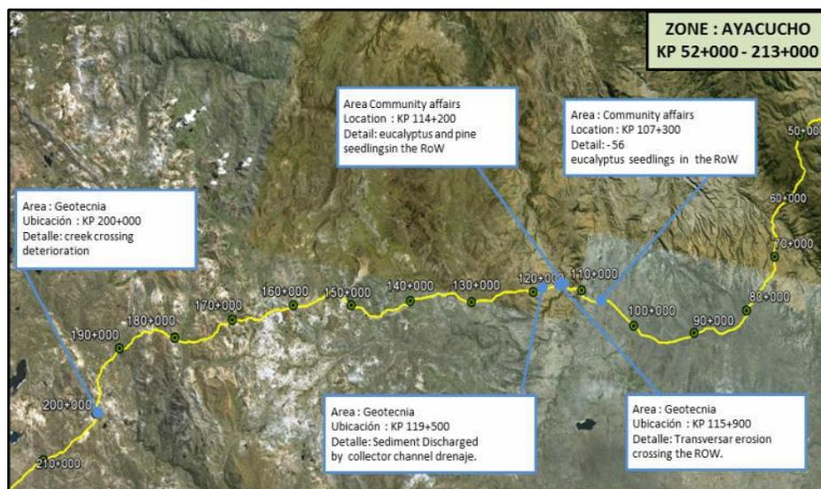
Figure 2 – PMSAP Findings recorded in the Ayacucho front in February 2012. The yellow line is the pipeline ROW.
